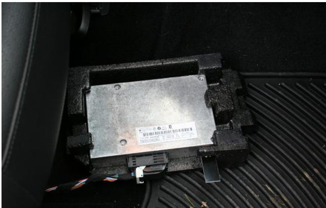
New controller with Bluetooth antenna ready to go back under passenger seat
